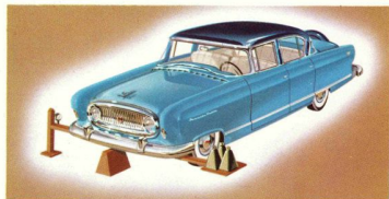
Torsion and bending tests by research engineers proved the 1955 Nash has more than twice the ordinary car's strength and rigidity. For example, it required 8,400 foot pounds to twist Nash one degree, less than half that, approximately 4,000 foot pounds, to twist the other cars (below) one degree.
