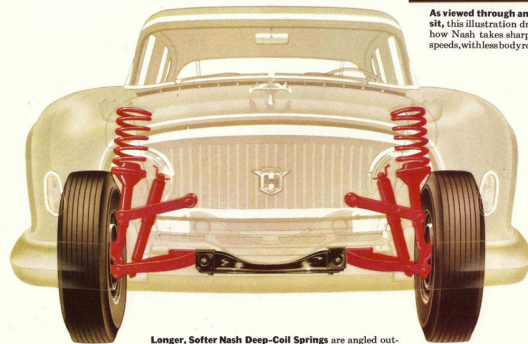
Longer, Softer Nash Deep-Coil Springs are angled outward like "Sea-Legs" for anti-sway control . . . lets you turn corners sharper and quicker than ever before.
