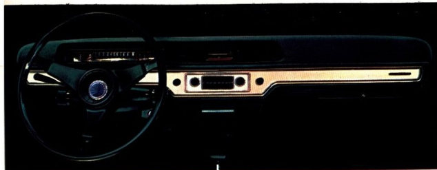
Controls for lights and wipers are located on the steering column in two large rotary switches. Of course, both the steering wheel hub and the instrument panel are completely padded.
