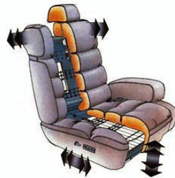
LX split bench seat illustration shown with optional leather seating surfaces and 6-way power seat adjustments indicated.
