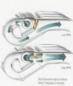
Induction Control system. Each cylinder draws air from two induction ports a long-and-thin port (top) for high-speed/low volume air instake at engine speeds below 3000 prn; and a short-and-wide port (botton) for high volume air instake at engine speeds above 4500 prn. Each cylinder draws from its two ports individually, or in combination, for maximum intake efficiency and frortied response, from diel to redline,
