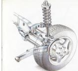
The rear wheels have been given a slight negative static camber so that side forces applied to the outside wheel during comering result in a relatively vertical wheel attitude, further improving fire contact with the road and enhancing the vehicle's cornering performance.
