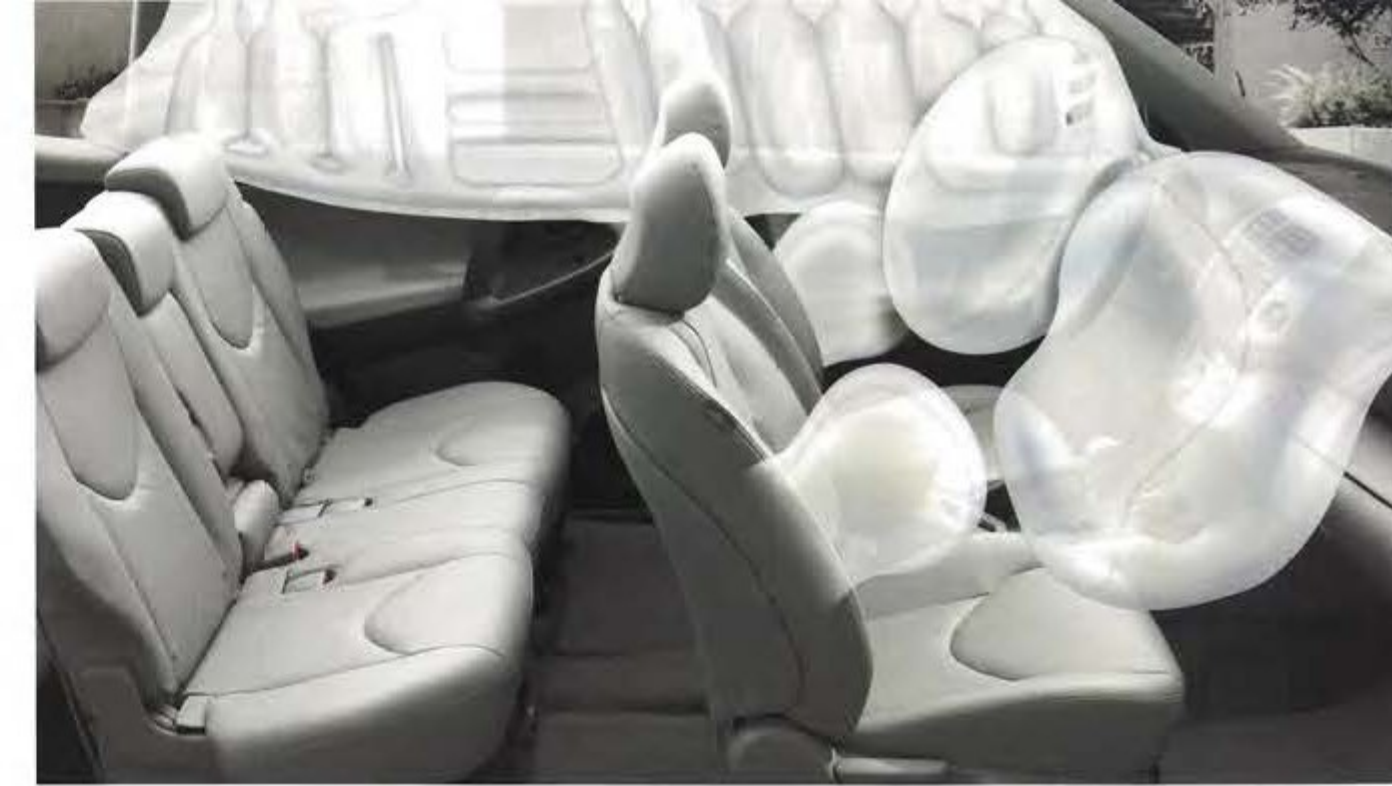
Available driver and front passenger front seat-mounted side airbags and front- and second-row roll-sensing side curtain airbags (RSCA). 1
