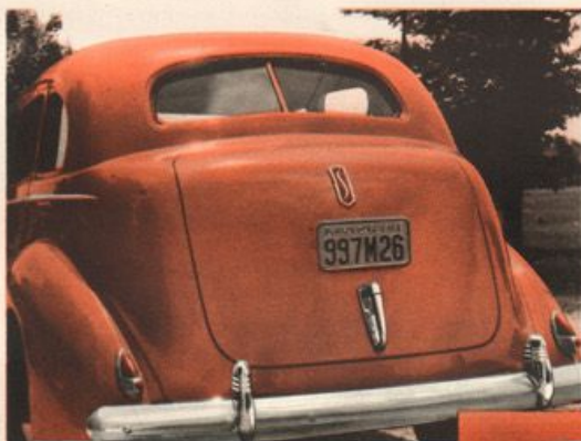
Door handles are streamlined with the stainless steel body belt in these new Studebakers—another distinctive Raymond Loewy touch that adds safety as well as beauty since the handles do not protrude.
