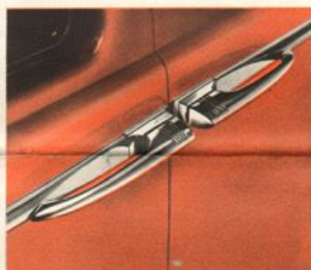
Door handles are streamlined with the stainless steel body belt in these new Studebakers—another distinctive Raymond Loewy touch that adds safety as well as beauty since the handles do not protrude.
