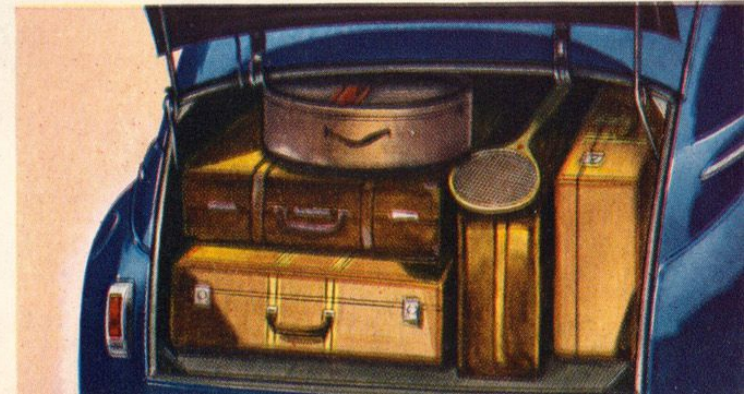
With the Ford's bigger, roomier bodies go big luggage compartments. Spare tire stands upright at back—out of the way—leaving room for plenty of luggage.
