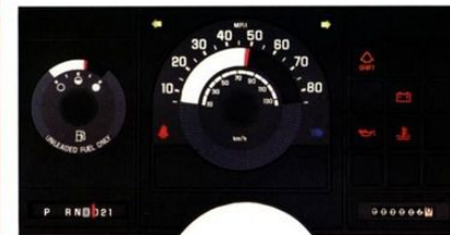
Cheyenne instrument panel with new, easy-to-read speedometer.
