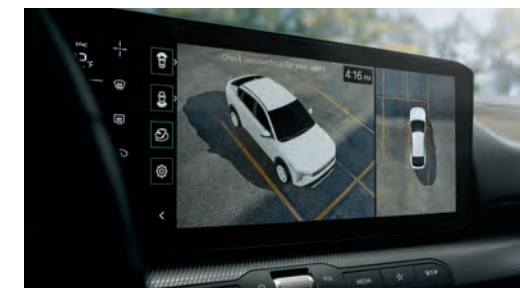
Surround View Monitor (SVM) 1,2 displays a 360° view of your surroundings to help enhance awareness when manoeuvring your vehicle in certain situations.
