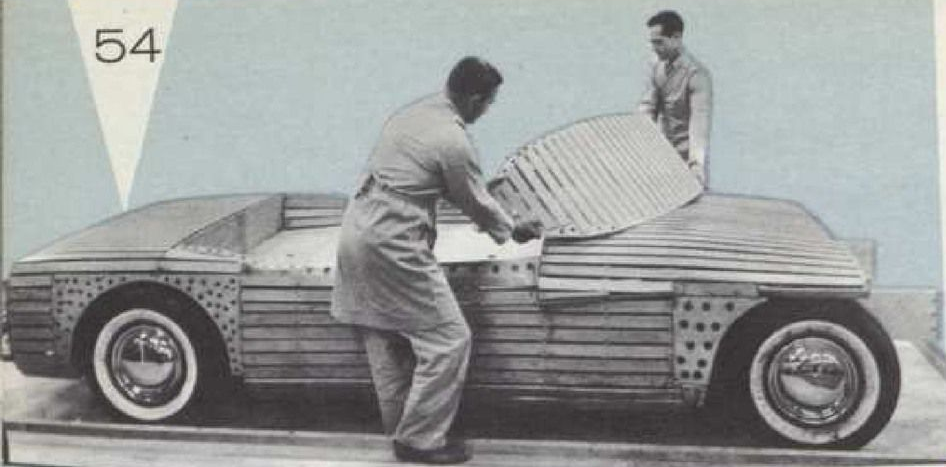
Clay modelers position windshield on wood armature. Slatted construction anchors clay.
