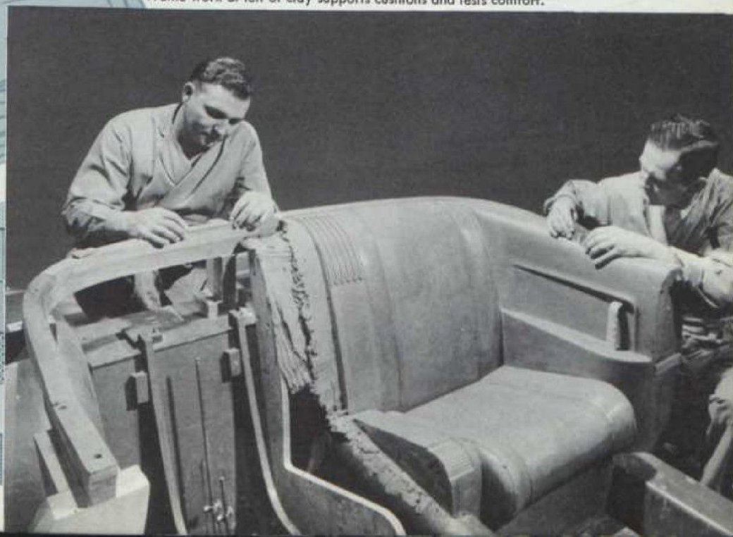
Clay mockup of back seat and rear inner quarter panel. Frame work at left of clay supports cushions and tests comfort.
