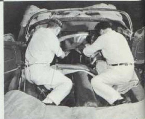
Floor covering is fitted to underbody prior to installation of seats.
