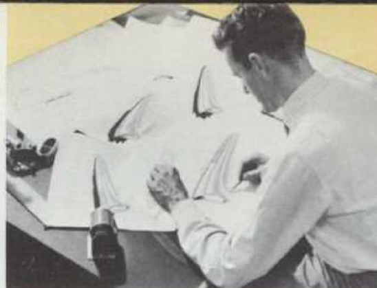
Several variations of a headlight detail are worked out by designer. Used in conjunction with a speed line that starts at the hood and merges with the sweep spear at the side (see below) this feature was later dropped.
