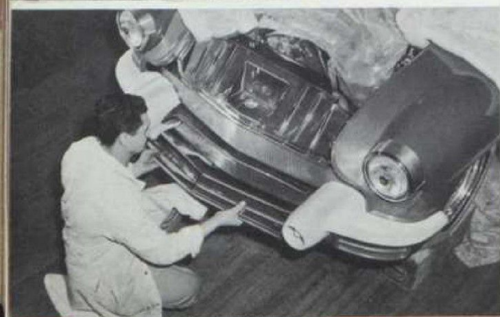
(Above) With the car almost completed, the plastic-coated windshield is fitted in place. Great care must be taken here to insure even pressure in the supporting molding. (At left) Chrome-plated bumper plate is positioned. Temporary white plastic covering protects other bumper parts.
