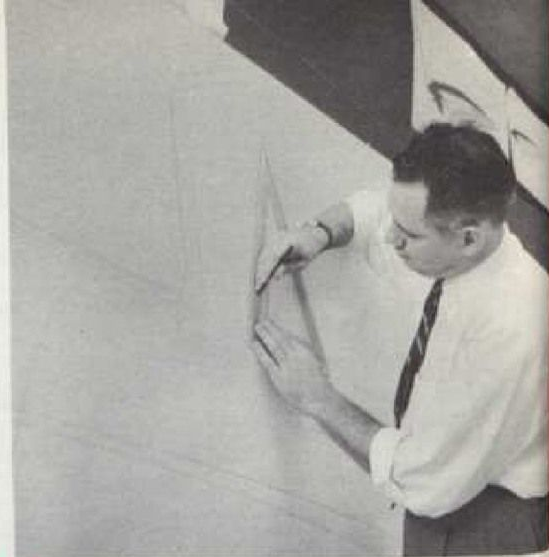
Designer converts small scale sketch into a full size line drawing. In the process he begins to develop and refine the design theme. Lines developed here are duplicated in wood templates and used to control the clay surface.
