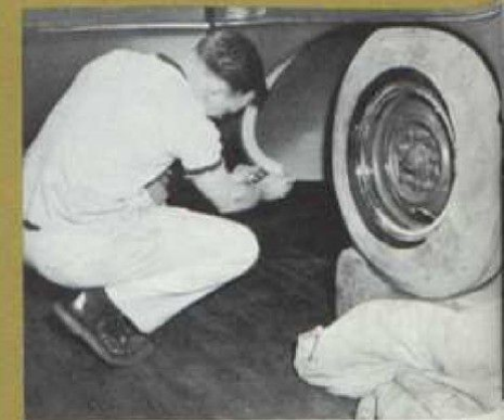
Painter prepares to touch up damaged paint. Note rubber boot on wheel. It will protect tire against damage during shipment.
