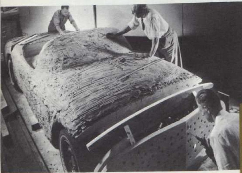
Clay heated to 150°F is applied with a thrusting motion to eliminate air bubbles.
