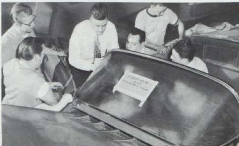
(Above) With the car almost completed, the plastic-coated windshield is fitted in place. Great care must be taken here to insure even pressure in the supporting molding. (At left) Chrome-plated bumper plate is positioned. Temporary white plastic covering protects other bumper parts.
