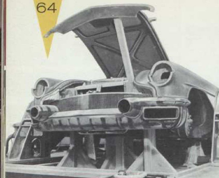
Up on blocks the partially assembled body (left) shows condition of Fibreglas before painting and brass metal before chrome plating. In the paint shop (above) a painter masks a fender in preparation for painting the underfender.
