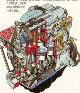
2.2 L max. power up to 64 DIN PS @ 4000 RPM. Max. torque up to 13.6 DIN kgm @ 2000 RPM.
