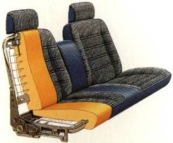
Lumina seats feature a new steel-spring suspension construction designed to provide better support and durability than seats of conventional full-foam design.
