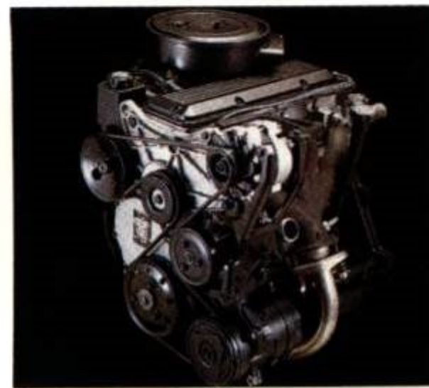
Standard 2.2 Liter L-4 with EFI 95 HP at 5200 RPM. Electronic Fuel Injection; crank-triggered, direct-fire ignition to eliminate periodic timing adjustments; low-restriction intake manifold; single belt accessory drive designed to never need tensioning.
