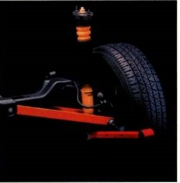
Lumina's sure-footed feel is due, in great part, to standard four-wheel independent suspension, four-wheel disc brakes and all-season radial tires.
