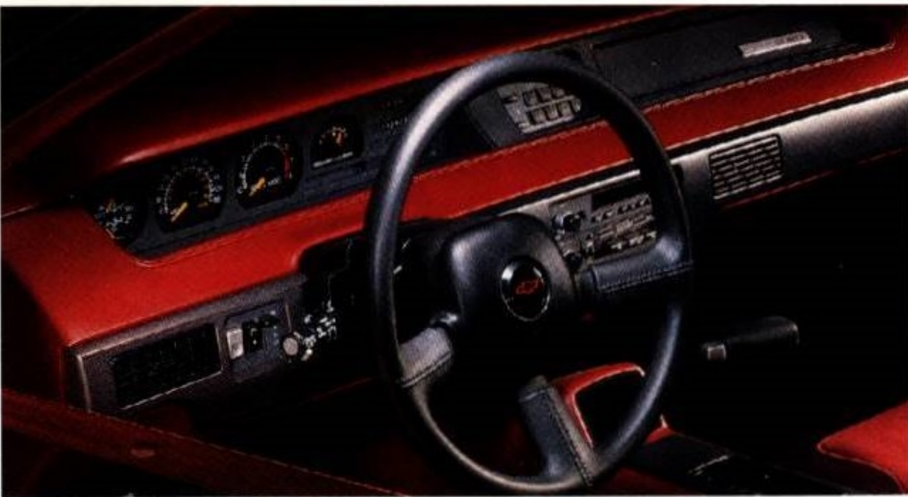
Lumina Euro instrument panel with optional gage package. Includes tachometer, trip odometer, oil pressure gage and temperature gage.
