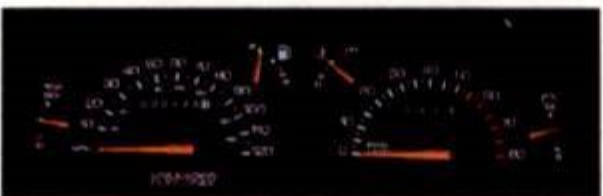
Gage package features analog voltmeter, temperature gage, tachometer and trip odometer. Standard on LTZ.
