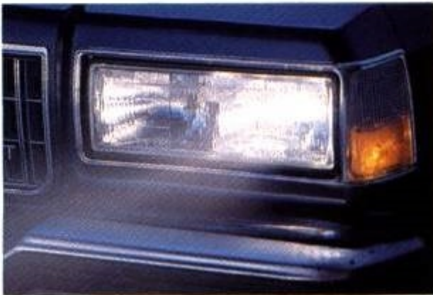
Composite halogen headlamps feature flush-fitting lenses and replaceable bulbs.
