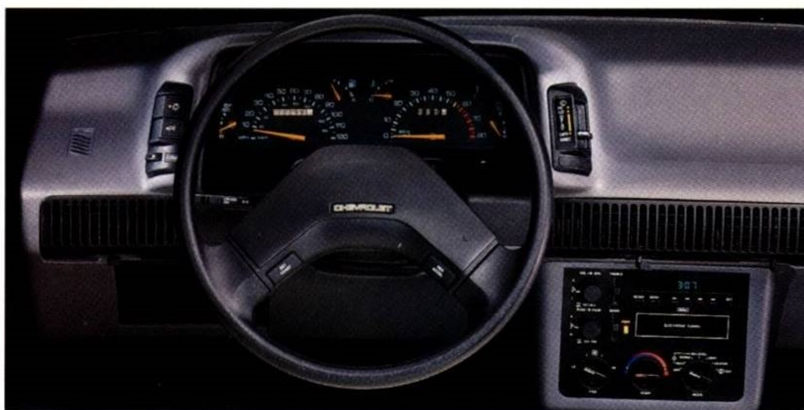
Standard instrumentation includes an analog gage package with tachometer, temperature and oil pressure readouts, voltmeter and trip odometer.
