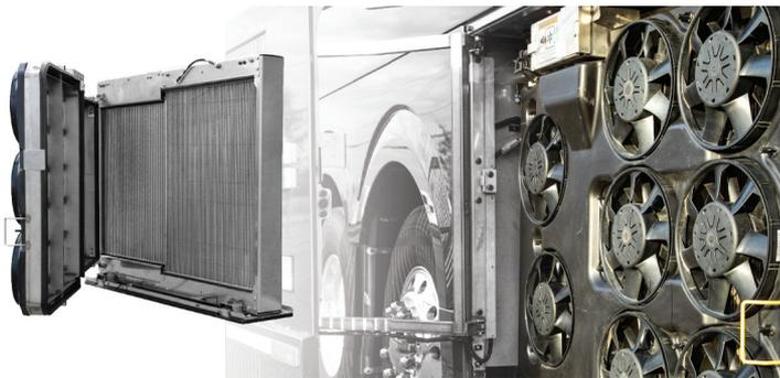
The side by side configuration allows the complete surface of both the radiator and the Charge Air Cooler (CAC) to receive fresh air. Debris cannot accumulate between them and the system logic was built with the following features to keep them clean and fully efficient at all time.
