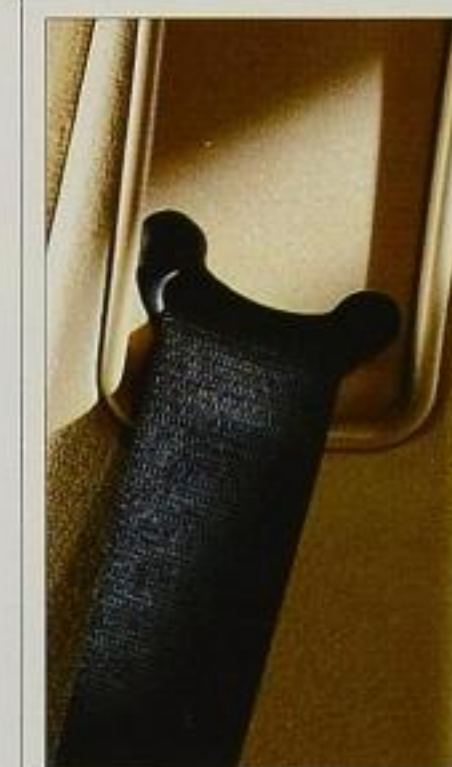
The top seat belt anchorage point of the front belts moves up and down automatically depending on seat position. Optimum seat belt geometry at all times without undue pressure on the body.
