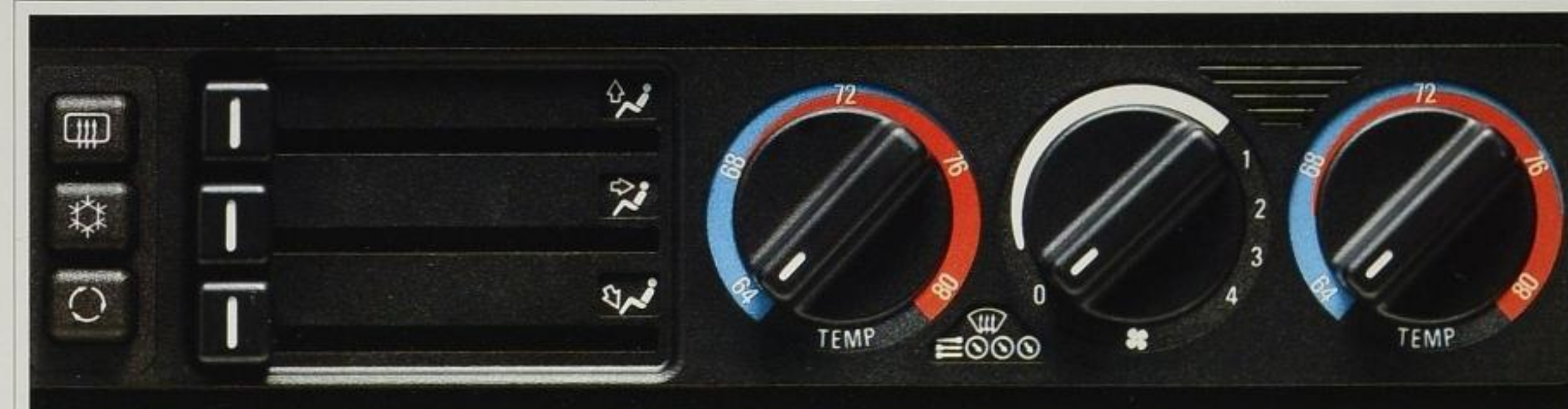
Electronically controlled heating/ventilation. Separate controls for the driver and front passenger. Perfect distribution of air. Extra-large, quiet, infinitely adjustable radial blower.
