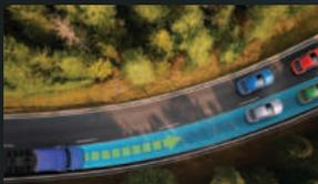
ABA6's expanded field of detection allows the system to detect vehicles in curves and issue warnings or automated emergency braking on them.
