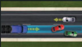
ABA6 now has the capability to recognize and respond to offset vehicles and those positioned at an angle, which is commonly seen in situations following an accident ahead.
