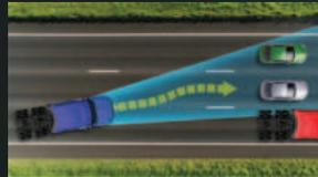
ABA6 can now detect vehicles in adjacent lanes. ABA6 allows the truck to respond if the driver swerves into those lanes at the last moment to avoid a collision in their current lane.
