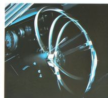
Tilt Steering Wheel adjusts to 7 selective positions. Affords up to 2 1/4" more entrance room.
