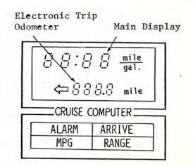
The operation of this sophisticated computer is controlled by a keyboard at the head of the center console, with the readout appearing on the instrument panel. The specifications of each function are detailed below:
