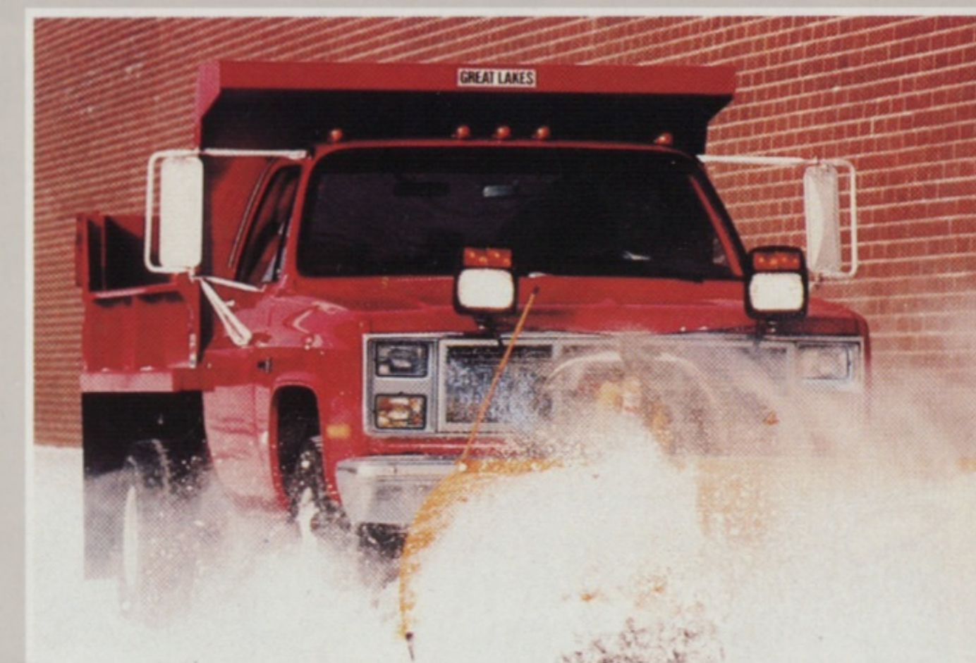
Sierra Cab & Chassis with available dual rear wheels. Dump body and snowplow are available from aftermarket equipment suppliers.
