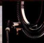
Continental's Anti-Lock Brake System begins with a speed sensor at each wheel that sends information to a microprocessor.
