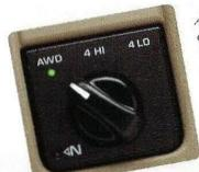
A new twist. Dodge engineers are always improving things: like taking the function of a floor-mounted transfer case shift lever and putting it into a convenient new electronic control knob – mounted right on the instrument panel.
