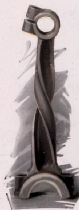
Ample evidence that Ford Vanadium steel connecting rods will never snap
