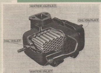
The Oil Temperature Regulator insures ideal lubricant temperatures under all extremes and greatly prolongs the life of the oil.
