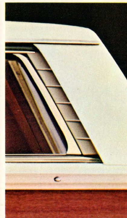
BUILT-IN AIR DEFLECTORS HELP CLEAN REAR WINDOW
