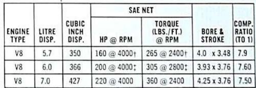
† 1-1-79 = 160 HP @ 3800, torque 275 @ 2400. † 1-1-79 = 190 HP @ 4000, torque 305 @ 2400.
