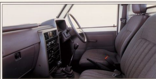
Convenient gear lever position for on-the-move changing. Cabin sealed against exterior noise and dust.
