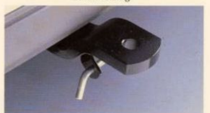
Towbars. Specially designed for Fairmont to comply with Australian Design Rule (ADR44) specifications.
