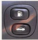
Remote release for fuel filler door and boot lid.
