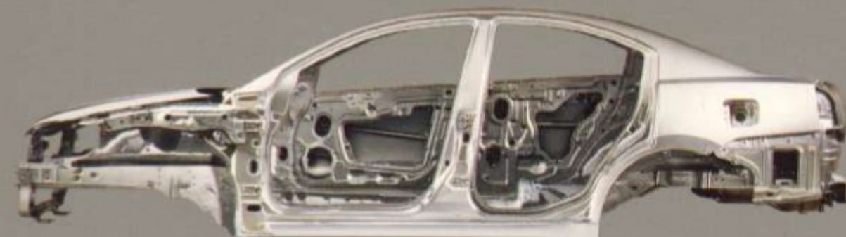
Mitsubishi Refined Impact Safety Evolution (RISE) chassis
