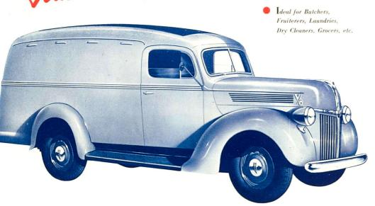
THE FORD V.8 15.18 CWT. 122 IN. W.B. VAN— This new model, designed for loads normally too heavy for the 112 in. W.B. Panel Van and too light to houl economically with heavier trucks, fills the want for larger van bodies for light bulky loads, giving in addition exceptional economy of operation. The broad side panels are admirably suited to every form of signwriting display and a good "game-plate" added to its hondsome
