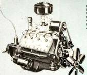
FORD V-8 LONG LIFE ECONOMY EN(NE developing 170 ft. lbs. torque and 95 E.H. Long life features for which this power unitras become famous include: Floating type co-secting rod bearings, mirrer finished cylinder wils, oil bath air cleaner, cast alloy crankshaft, e.
