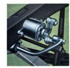
LIKE A GIANT'S HELPFUL HAND, the newly-designed, perfected ride-stabilizer restrains body sway or swing on curves and rough roads, makes steering easier, adds to riding comfort. New soft transverse springs and double-acting shock absorbers gently take up road irregularities.
