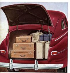
CONCEALED beneath the smooth rear deck is a yasming luggage compariment large enough for a whole family's baggage. Spare wheel and tire are stowed vertically against the wall; floor mat, light that turns off and on automatically, and tools are standard equipment in all cars. Luggage is protected by a safety lock that holds the key until the compartment is locked. Combined tail and stop lamps are set flush with body. Note the generous width of the Mercury body all the way up.
