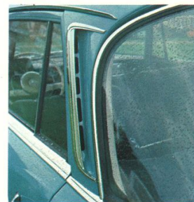
Rear ventilators exhaust interior air
