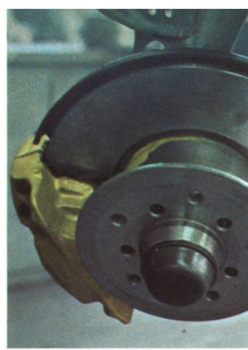
Fade-free caliper-type front disc brakes
