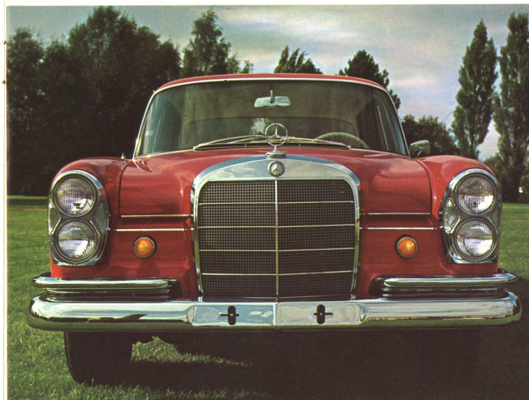
Radiator grille has remained virtually unchanged since 1912. The body design was established by wind tunnel tests and contributes to quiet at high speeds.
