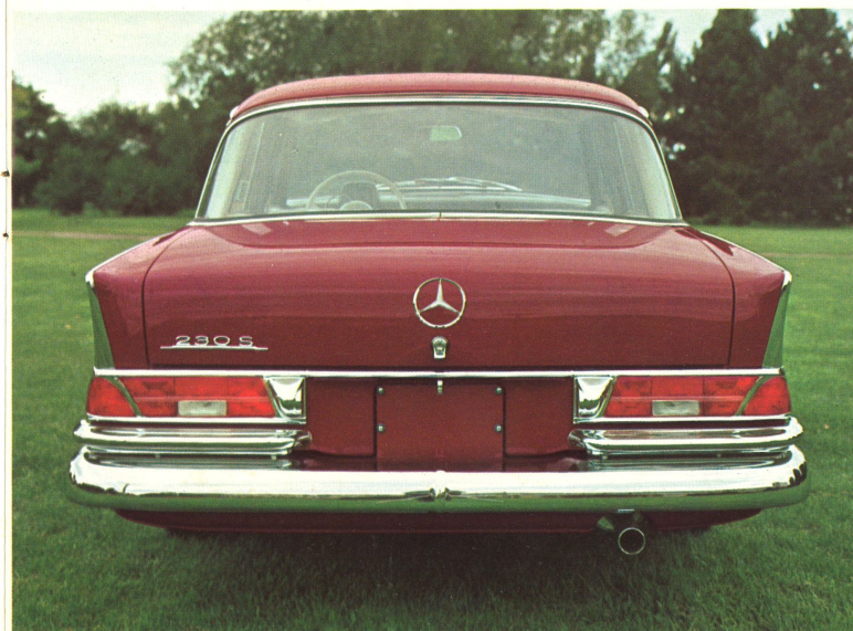
Brake, back-up and turn indicator lights are combined in single units. Gas filler cap is behind hinged license plate door. The spacious trunk holds 22.6 cu. ft. of luggage.
