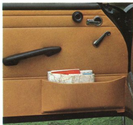
Front door features map pocket, recessed handle, padded window crank and armrest
