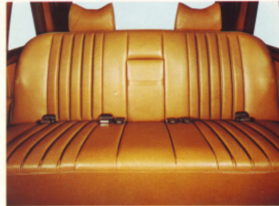
Three-point safety belts for the front seats and lap type for the rear seat, comfort headrests.
