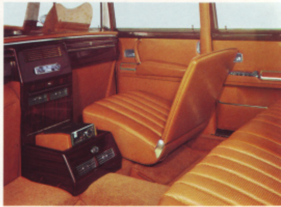
6-door, 7-passenger sedan with partition wall, air conditioner, tape recorder and radio remote controls
