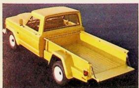
A brand new 120" wheelbase model, rated at 6000 GVW, has just been added for 1972. It's also available with 5000 GVW rating. The 132" wheelbase model is available with a 5000, 6000, 7000 or 8000 GVW rating. The 8000 GVW model is specially designed to handle big, roomy cab-over camper units under the most demanding highway and offroad conditions.
