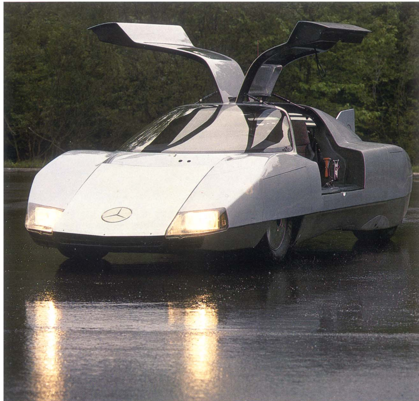
1978. C-111-3 research car, powered by a turbocharged 3-liter Diesel engine, averages 195.39 mph in setting 9 new world speed records—and delivers 14.7 miles per gallon.
