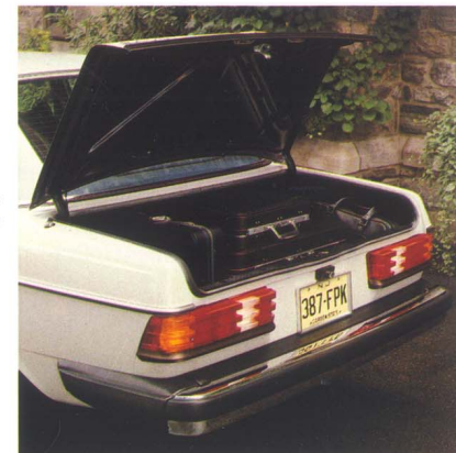
The trunk has 12.57 cubic feet of unobstructed luggage space. The spare tire and tool kit are tucked away beneath the floor.
