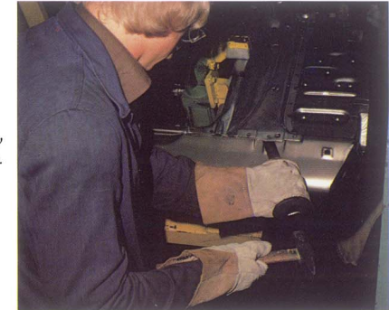
Inspectors continuously check body welds for strength.
