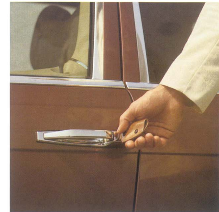
The convenient central locking system: one turn of the key or one push of the lock button on the driver's door, locks the doors, the trunk, even the fuel filler port.
