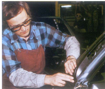
Weather sealing materials are carefully applied to window frames, doors, and trunk to assure a watertight interior.
