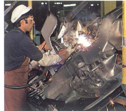
Connecting body panels are carefully welded, soldered, and ground smooth to eliminate any trace of a seam on the body finish.
