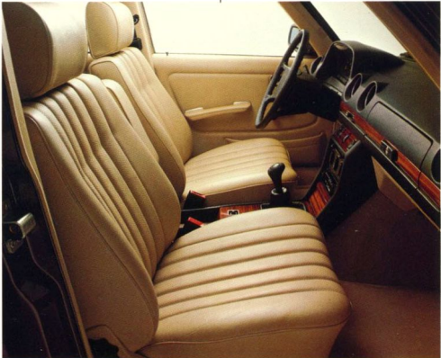
Front seats employ several padded layers over a steel spring core, for firm but supple body support.
