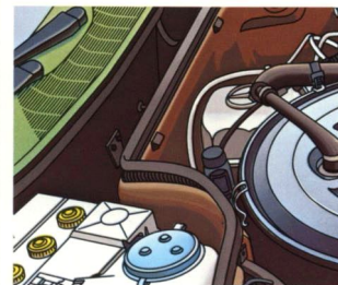
Ingenious "double firewall" acts to further muffle engine noise.
