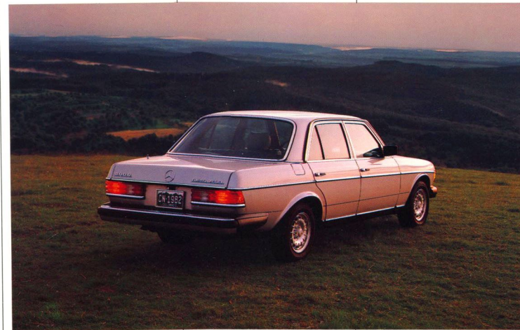
300D's silvery, forged light-alloy wheels dress up its appearance, while cutting unsprung weight.
