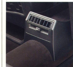
This ventilation console is placed in the cabin expressly to serve rear seat passengers.
