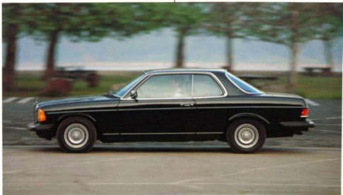
300CD bodywork is not just a handsome coupe form. It is also an aerodynamically efficient wedge.
