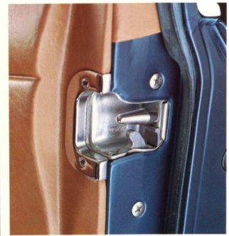
Mercedes-Benz door locks are so strong that any one could take the weight of the entire car.
