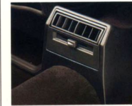
Separate ventilation console is provided for rear passengers in 300SD, 380SEL, 380SEC.
