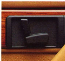
This seat-shaped control electrically adjusts your seat position; just touch its corresponding part.
