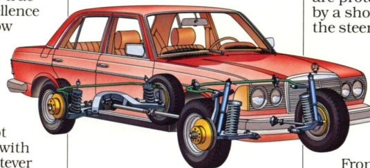
Mercedes-Benz suspension is designed to combine riding comfort with handling stability.
