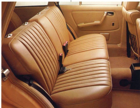
Sections of split rear seat can be separately folded down to create instant cargo space.
