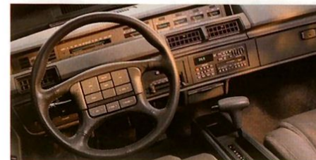
The S/E instrument cluster features a Driver Information Center, analog speedometer, tach, fuel, coolant temperature and oil pressure gauges plus voltmeter.
