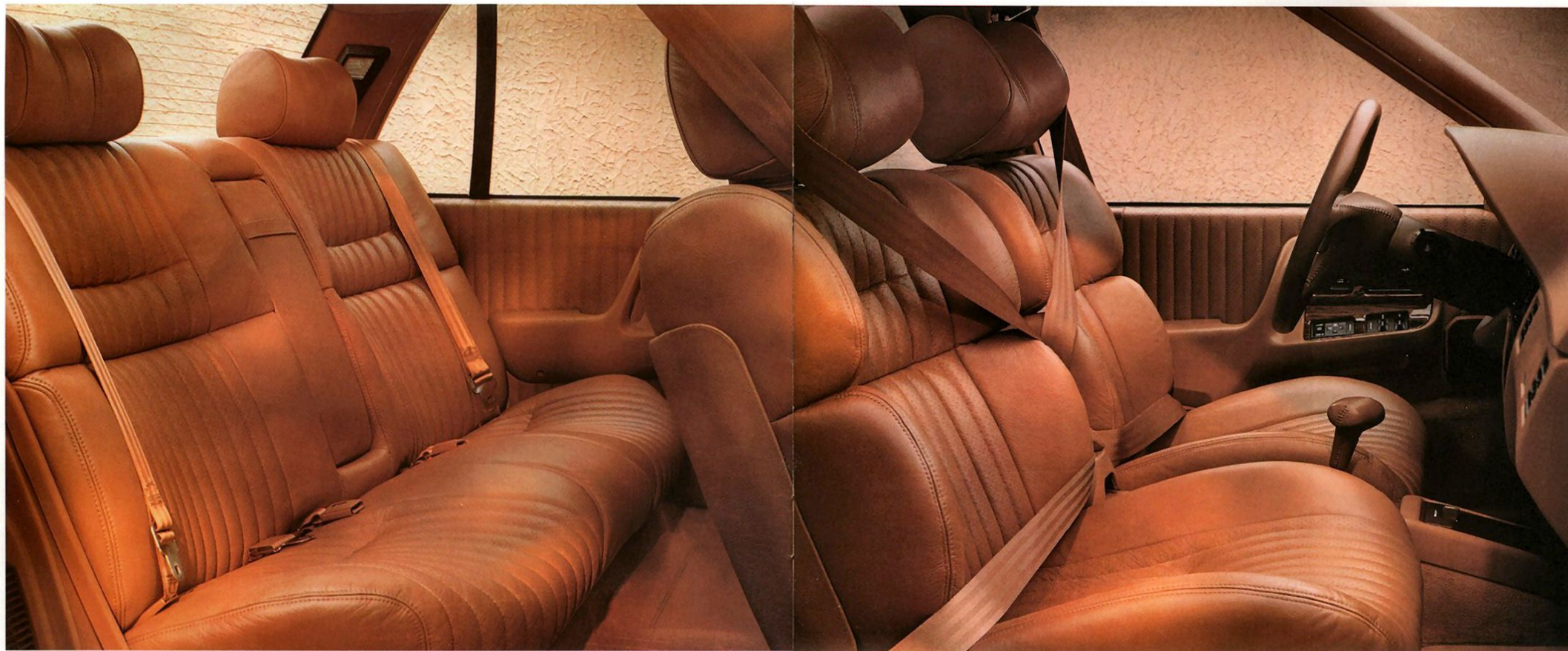
SSE's three lumbar supports can be inflated at the touch of a button to support your lower back, while the headrest can tilt in or out.
