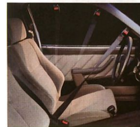
The GSE has specific, highly bolstered Sport seats that are complemented by a new, automatic passive-restraint safety belt system.
