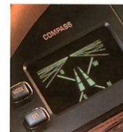
SSE's electronic compass has four built-in corrections for the difference between magnetic and true north as you traverse America the Beautiful.
