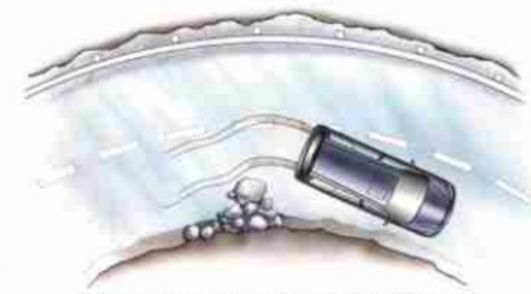
Anti-lock brakes can help the driver retain steering control during hard braking.
