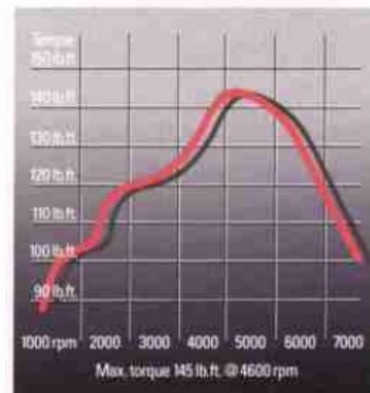
The 2.2 liter Odyssey engine produces plenty of torque over a broad range of usable engine speeds.
