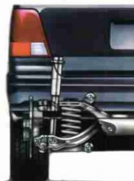
Compact double wishbone rear suspension gives the Odyssey stable handling and a smooth ride, yet takes up minimal space.
