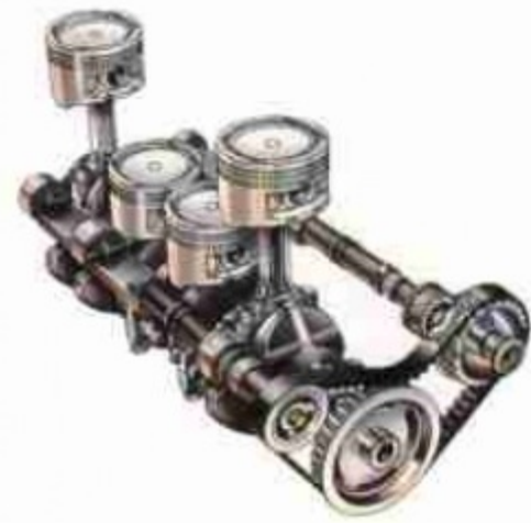
The Honda-designed second-order balance system helps minimize engine vibration.
