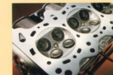
▲ FORMULA ONE RACING-INSPIRED 4-valve-per-cylinder design delivers impressive performance in the city and on the open road.
