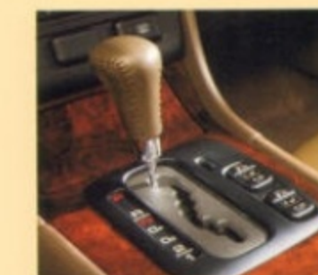
▲ THE GATED SHIFTER of the 4-speed automatic transmission gives a more intuitive response and a more positive feel.
