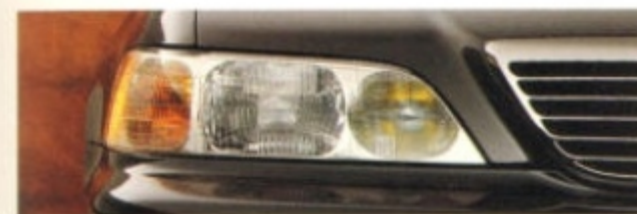
▲ The headlights of the RL switch on and off automatically, according to the outside light level.
