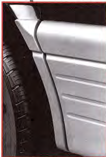
Lower bodyside cladding helps to resist chipping and denting
