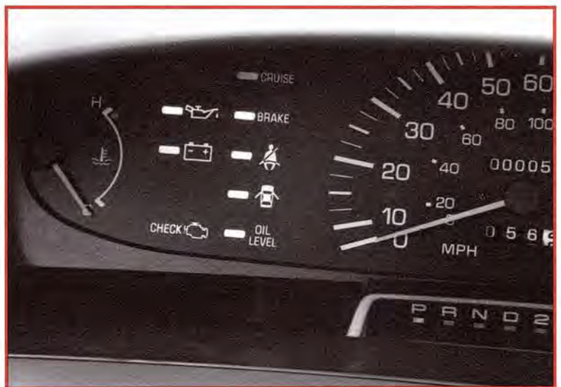
Warning lights are shielded from glare and thus are easy to see
