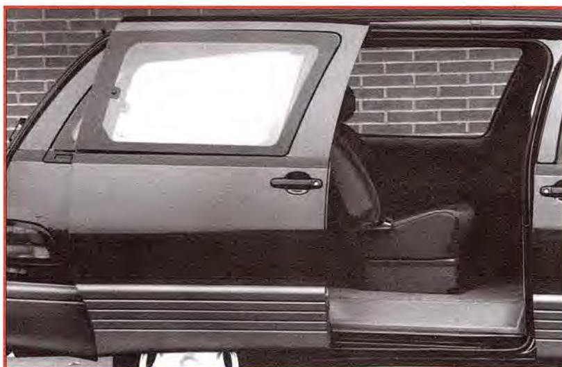
The Previa's easy to operate sliding side door opens only to the curb side for safety reasons
