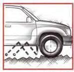
Anti-chip paint reduces stone damage
