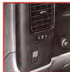
The push-button clutch start cancel switch is conveniently located on the lower left of the instrument panel
