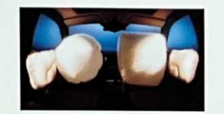
Brake Assist and BabySmart\* expand upon two safety features found in every Mercedes passenger car—an Antilock Braking System (ABS) and air bags. Brake Assist senses emergency braking by the speed and force of the brake pedal application, and automatically delivers all available power brake boost—more quickly than the average driver might—until the pedal is released. Resulting in potentially shorter stopping distances.
