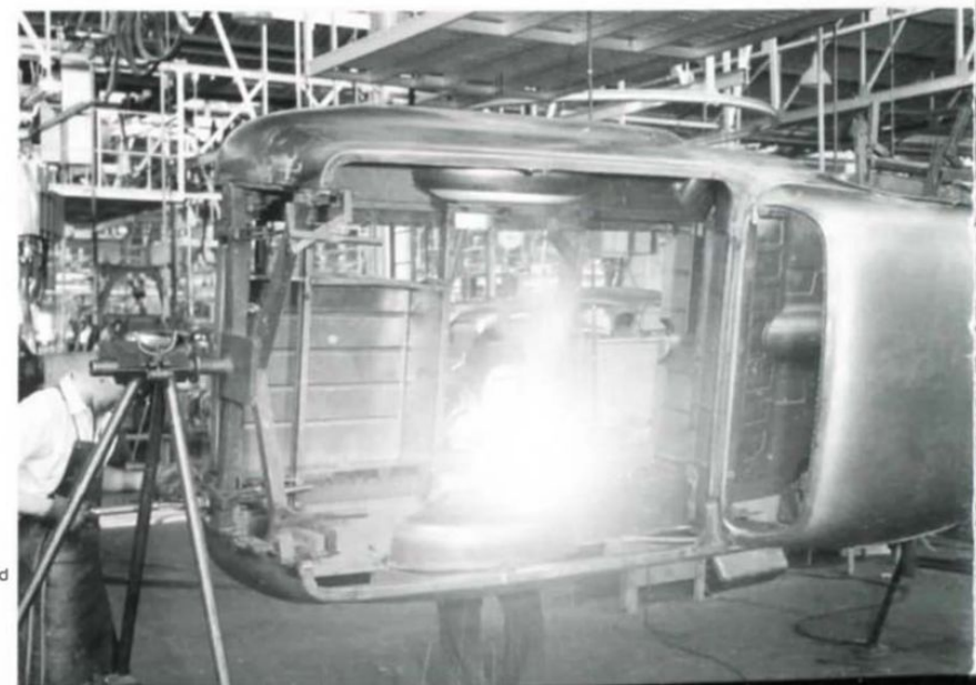
January, 1951. Long before the days of robot welders, one of the first 50-2106 Ute bodies produced undergoes the welding process, mounted on a special jig.
