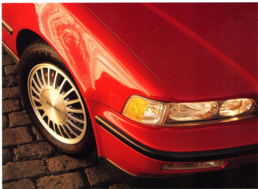
THE AGGRESSIVE FLAIR OF THE FRONT FENDER IMPROVES AERODYNAMIC FLOW BY REDUCING TURBULENCE AT THE WHEELWELLS. THE CAST ALUMINUM-ALLOY WHEELS REDUCE UNSPRUNG WEIGHT FOR IMPROVED RIDE QUALITY AND MORE PRECISE HANDLING.
