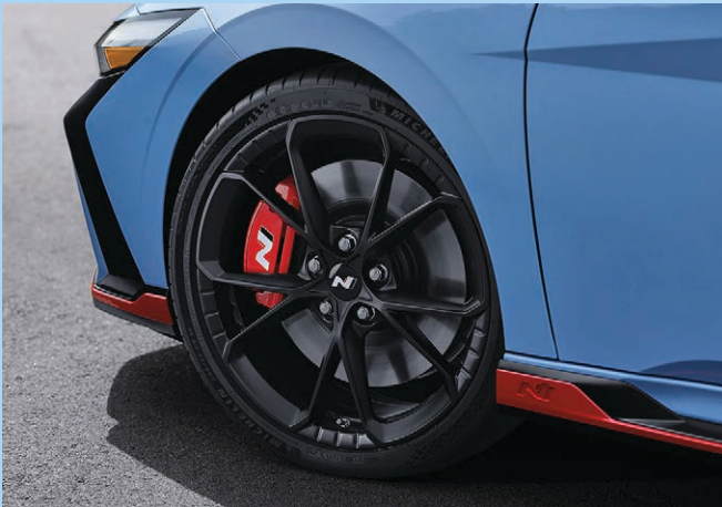
19” forged wheels and 14.2” front brake rotors
