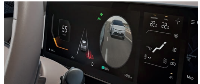
Blind view monitor displays the blind spot in the direction your turn signal is indicating.*
