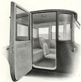
Interior of the Coupe. The auxiliary seat may be folded under the cowl.
