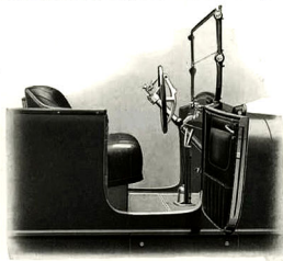
Showing hinged steering wheel, dropped, permitting easy entrance and exit at either side for front seat passengers
