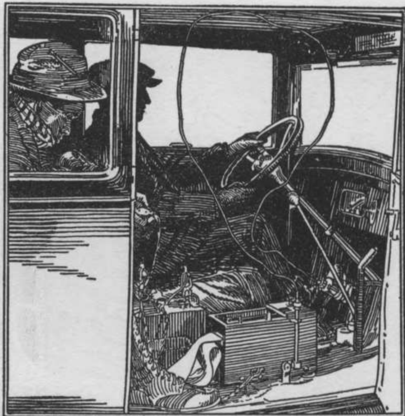
Measuring brake pedal pressure and deceleration
