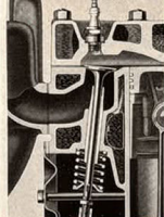
Angle set valves for combustion efficiency
