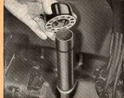
Forced-draft crankcase ventilation removes all harmful oil vapors from the engine
