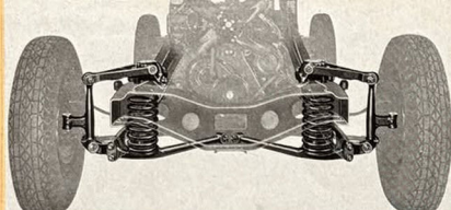
The Packard SafeTflex front wheel suspension gives a far softer ride, positive wheel alignment, maximum tire life and freedom from adjustments
