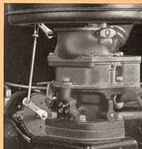
The automatic choke makes starting easy on the coldest day
