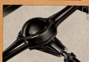
Packard's exclusive Angleset rear axle allows lower set bodies with head-room maintained
