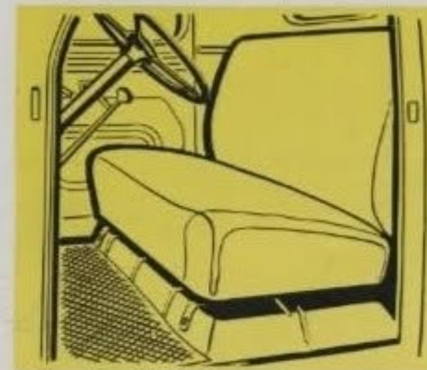
The manually controlled lever allows a three-inch seat adjustment, a feature much appreciated by drivers. In this view the seat is in rear position.
